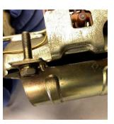
Take the fuel hose and carefully fit over the output pipe on the fuel cradle. This may need a
