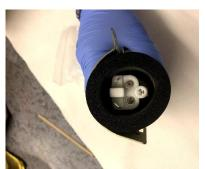
By carefully pulling down the foam isolator to expose the fuel pump output, fit the supplied rubber submersible fuel hose onto the output barb and use one of the supplied pipe clips to secure the hose to the pump.
