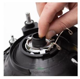
Step 6: Insert the bulb holder into the headlamp unit as pictured, with the black cylinder facing outside.
