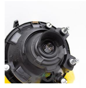
Step 1: Unplug the headlight wiring from the back of the headlight by gently pulling on the connector (do not pull on the wires directly as you may cause damage to the headlight wiring).
