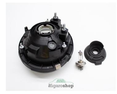
Step 3: Remove the old headlight bulb from the headlamp by pinching the two metal retaining prongs and pulling away, this will leave the bulb loose in the holder. Then gently remove the bulb, take care when putting aside as the old bulbs are very fragile and can break easily.
