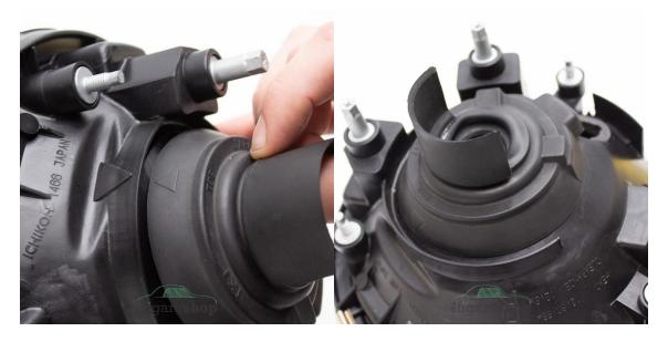
Step 9: To install the bulb into the headlight line up the two pins on the bulb with the matching points on the holder, push in and twist clockwise to ensure they are locked into position. Once fitted the wires should come out pointing towards the bottom.
