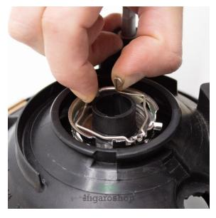
Step 7: Secure the bulb holder in place by pinching the retaining prongs and locking into place (just how it was before removing the old bulb.
