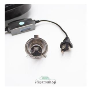
As you can see the new LED headlights connect to your car with the same 3 pin H4 bulb connector.
