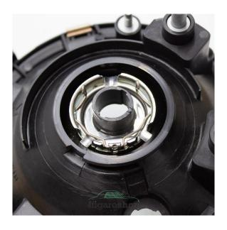
Step 8: Place the headlight seal over the bulb holder and ensure that the two triangles on the headlight and the seal line up correctly. Press the seal onto the headlamp and ensure it fits securely.
