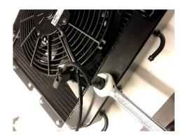
• Bolt the resistor pack using the supplied m6 bolts to the new radiator with a 10mm socket and ratchet in the orientation shown below and plug the fan switch into the loom as shown.
