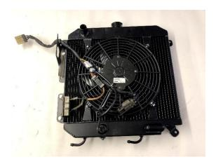
Reinstall the radiator, fill and bleed the coolant system and ensure the fan switches on and off when needed. You can now enjoy the peace of mind that you have installed the very best in cooling performance for your Figaro.
