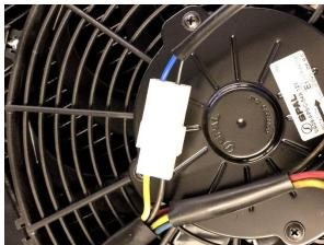
• You are now nearing the final steps of the installation. Ensure the plugs of the fan are secure and with 3 or 4 cable ties, fasten the loom to the casing of the fan making sure that the ties do not touch or interfere with the rotation of the cooling fan blades. Once this is done, you can finish your installation by bolting the coolant over flow bracket back onto the new radiator using the supplied m6 bolt in the top corner of the radiator.
