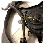
• The loom can now to lifted off the original fan to be used in the next steps of the guide.
