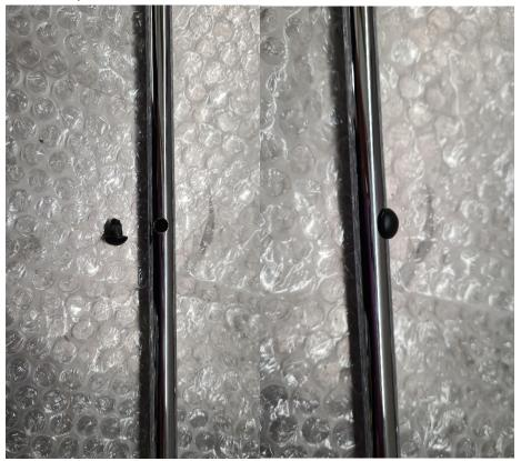
10. Screw the parking stick into the main chrome parking stick bracket all the way down. Once seated, rotate backwards to align the parking stick correctly. Once in the correct orientation, screw the chrome nut back down to tighten against the washer and main bracket to secure the parking stick.
