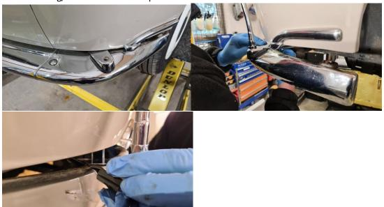
6. Un bolt the bumper bolt attaching the corner bumper to the centre bumper section and replace the bolt with the new genuine bolt included. Using the new nut, attach the under
