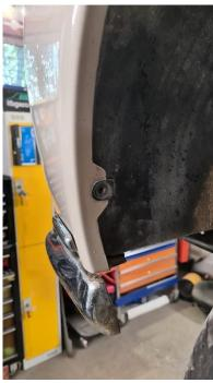
2. Bend the wheel arch liner away from the underside as shown so full access is available to your working area.
