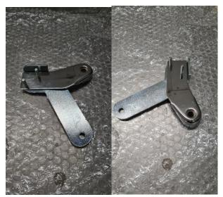
5. Fit the parking stick rubber isolator to the main parking stick bracket and slide it between the front wing/fender and the bumper as shown below
