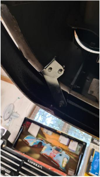
7. Re attach the bumper to the wing/fender re-using your old hardware. The main bracket should feel secure and fit snug between the wing/fender and the bumper.
