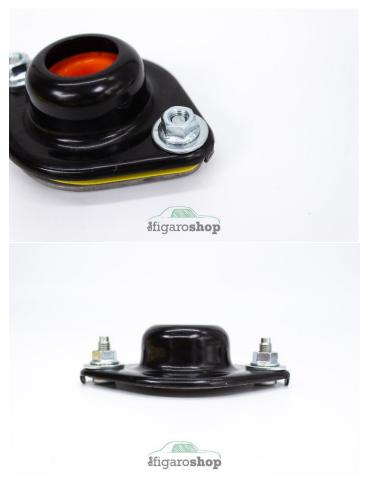
7. Once tight, turn the mount upside done once again, place on the cloth and using a small hammer, bend the tabs carefully back to their original orientation to secure both halves together.
