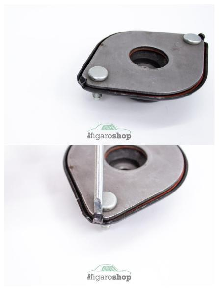
3. Once the tabs are bent up, remove the lower half from the upper half, remove the oval gasket and original rubber top mount insert.
